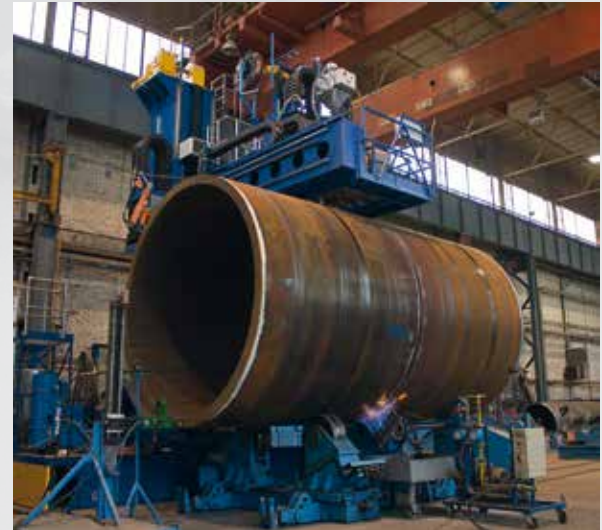
Machining of stiffened tubesheet system Robot welding
