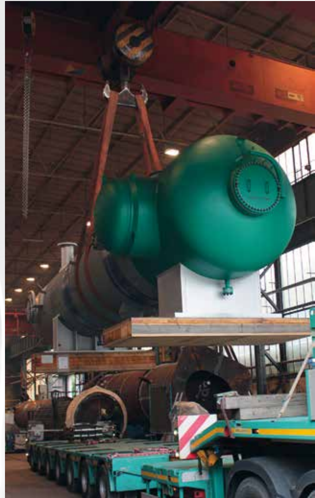
Waste heat boiler ready for shipment
