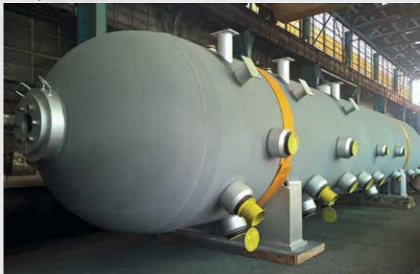
Loading of a steam drum
