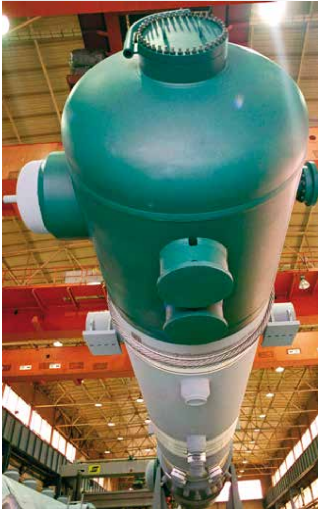
Process gas waste heat boiler
