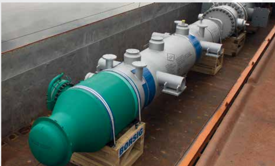
Waste heat boiler at the Borsig-Harbor
