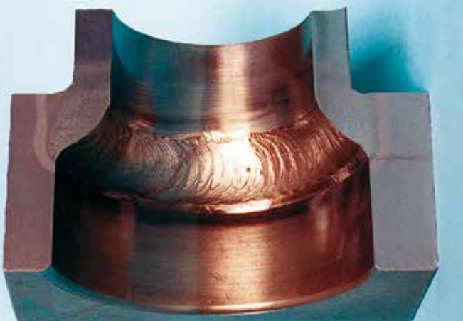
Specimen of tube to tubesheet weld
