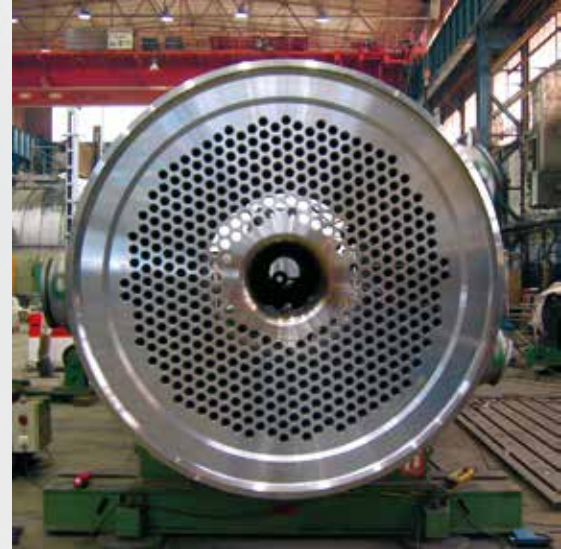
Gas inlet tubesheet with central bypass tube
