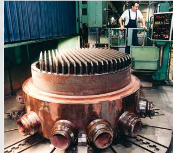
Machining of stiffened tubesheet system
