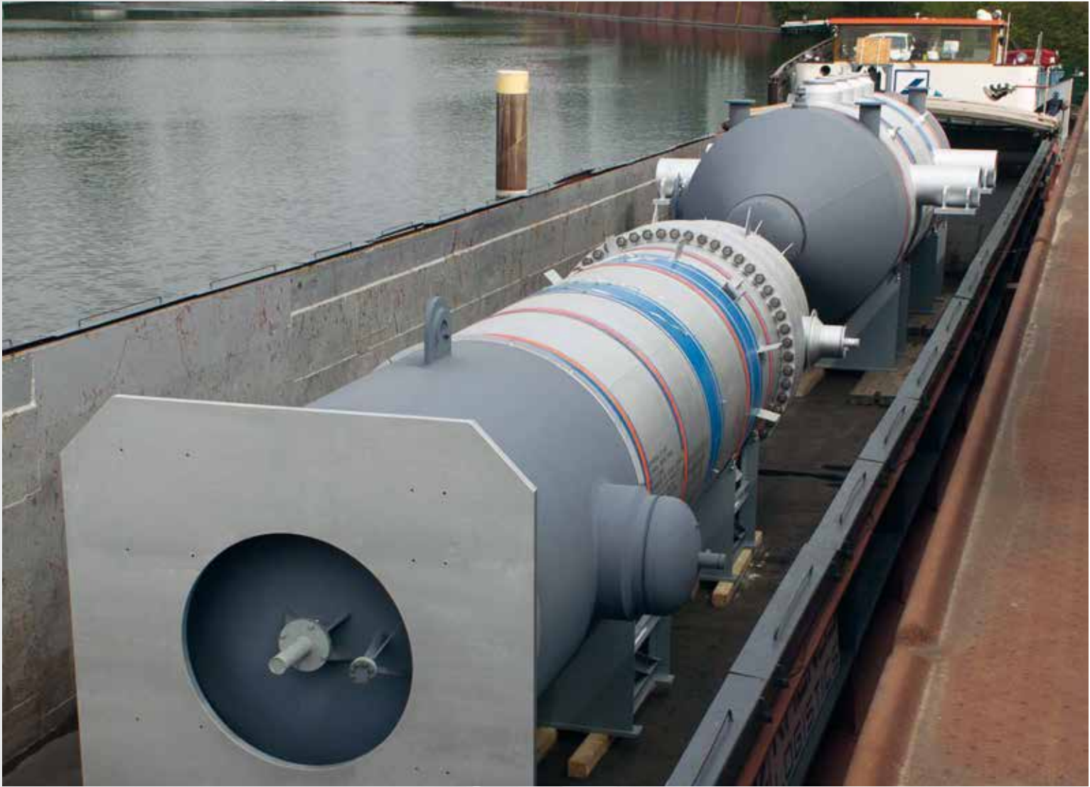
Borsig harbor: Shipment of a steam superheater
